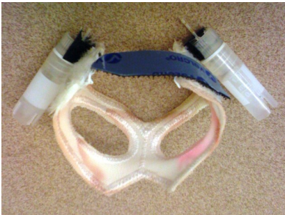
Custom built harnesses with attached cryovials that are used as receptacles for the urine from each individual rat ureter.
