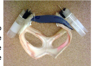
Custom built harnesses with attached cryovials that are used as receptacles for the urine from each individual rat ureter.
